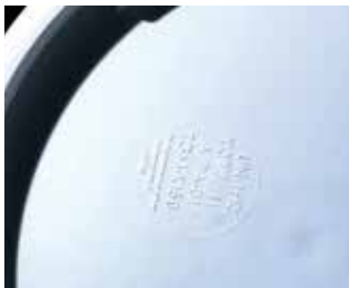
Lid with gripping lugs + UN labelling
